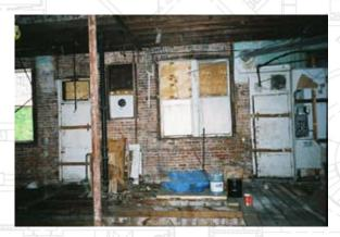
Existing Condition: 3,000 sq. ft. single story masonry building. The building was lacking floor, ceiling, and storefront constructions. Sorce Architecture designed and prepared drawings for all aspects of the new building, including restoration of the building, kitchen design, interior design, and bar/seating area layout. Sorce Architecture worked in close collaboration with the owners to achieve a successful design contributing to a successful business.
